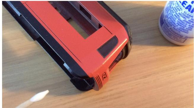
9. Test the fitting of the windshield. If it is not enough or too much round, bend it carefully. Verify that the upper part of the frame, the place of the destination sign, is painted black
