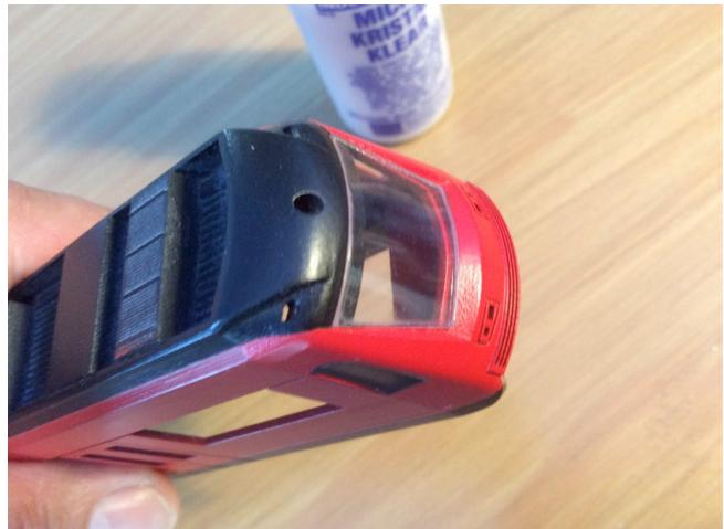
11. If using a functional pantograph, you have now to connect a wire to the metal screw provided by Sommerfeldt. The best way is using a brass washer with a solder tab. (When using the dummy pantograph, plug it only in the end after the following steps.)
