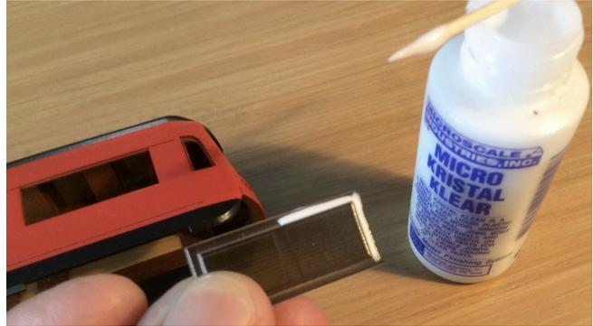
7. Let dry, and continue with the next window on the same side. Check the alignment, the windows have some play and can easily be aligned. Finish one side before starting the opposite range.
